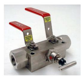
Machined from a barstock body, this valve features two inline ball pattern primary and secondary isolating valves and a needle vent valve.
