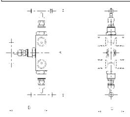
The 'Y33' and 'YV33' Type 3 valve manifolds are designed for remote mounting to differential pressure transmitters, with separate isolation for LP and HP inlets plus equalising valve for simple calibration. Each needle valve head is designed for safe and reliable isolation, giving bubble tight shut off, with non-rotating & anti-galling tip and dynamic self-adjusting spindle seal to give long service life in a variety of service conditions.
