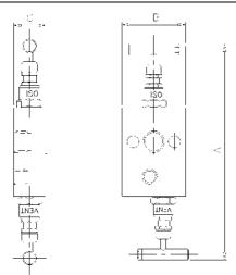
The 'Y24' and 'Y25' Type 2-valve manifold is designed for direct mounting to static pressure transmitters. The separate vent valve gives full control of venting of the instrument, plus the ability to calibrate in-situ. Each needle valve head is designed for safe and reliable isolation, giving bubble tight shut off, with non-rotating & anti-galling tip and dynamic self-adjusting spindle seal to give long service life in a variety of service conditions.
