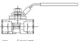
These high performance quality ball valves are stocked in 316 stainless steel. Even the pressed handle on the valve is 316 stainless steel to avoid rusting on site.
