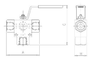
The 'B6BL' Type 3 way Flow Diverting Ball Valve is designed for safely diverting flow to one of the two outlet ports. Totally enclosed soft seats offer both positive sealing and low operating torques, from vacuum to high-pressure service. Anti-blow out spindle is fitted as standard with the PTFE spindle and body seals.
