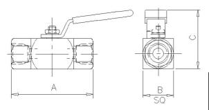
The 'B10' Type Single Isolating Ball Valve is designed for safe and reliable isolation giving bubble tight shut off. Totally enclosed soft seats offer both positive sealing and low operating torques, from vacuum to high-pressure service. Anti-blow out spindle is fitted as standard with the option of PTFE or Grafoil seals.
