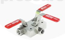
Barstock body with three balls arranged for sampling, chemical injection and double block and bleed of instrument. Surface mounting option available
