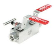
Barstock body with ball pattern isolate and secondary isolate valve and needle pattern vent.
