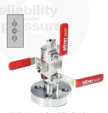
Machined from a single piece 'grain flow controlled' forging. This valve features two inline ball pattern primary and secondary isolating valves with ball valve vent, offering 'through to process' rodding in bore sizes from 10mm to 14mm (0.4'' to 0.55'').
