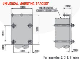
For mounting 2, 3 & 5 valve manifolds to a 2" NB pipestand. Mounting brackets supplied with "U" bolts, washers and nuts. Material of all components is zinc plated and passivated Carbon Steel. Special brackets can be supplied on request.
