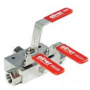
Barstock body with three balls arranged for sampling, chemical injection and double block and bleed of instrument. Surface mounting option available. Cam Interlock option available to allow only the correct sequence of operation and to prevent accidental opening of the vent valve when the first isolation valve is open.
