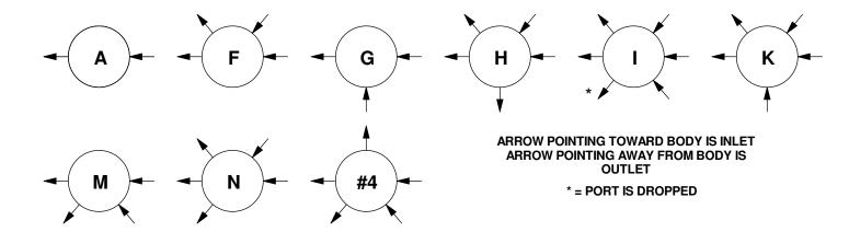
REFERENCE CLOCK 90° LOCATION OF PORTS VIEWING FROM TOP OF FIRST STAGE **DUAL STAGE PRESSURE REDUCING**
