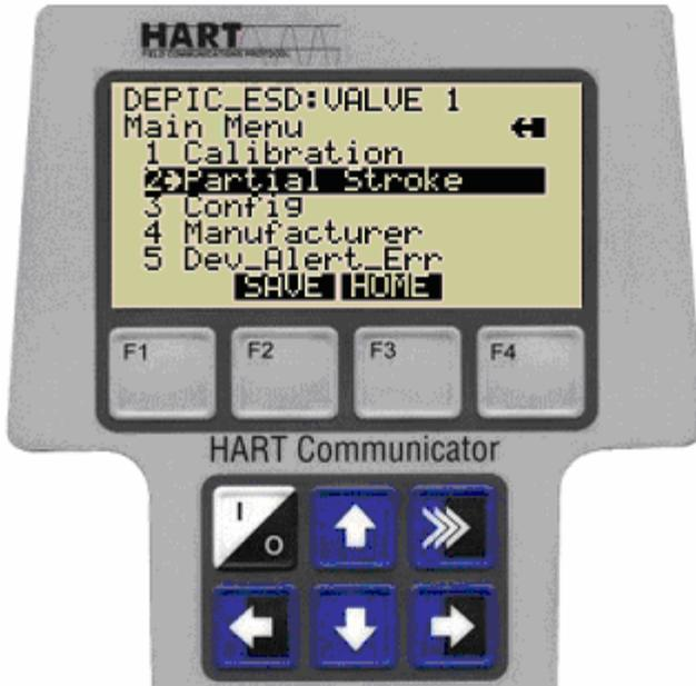
7.2.4 Start Partial Stroke by pressing → Key on 1.
