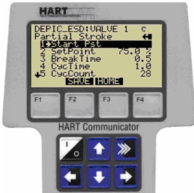
**7.2.5** Partial Stroke process can be continued by pressing F4 (OK) Key or can be aborted by pressing F3(Abort)Key.
