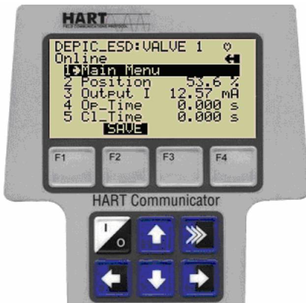
7.2.3 Select Partial Stroke by pressing → Key on 2.
