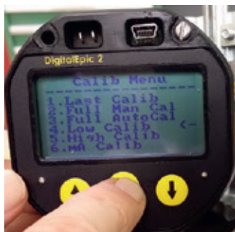
FIGURE 63 Accessing low calibration
