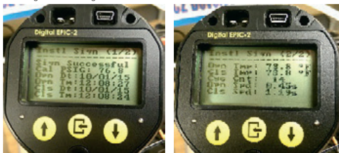
FIGURE 81 Viewing installer signature data
