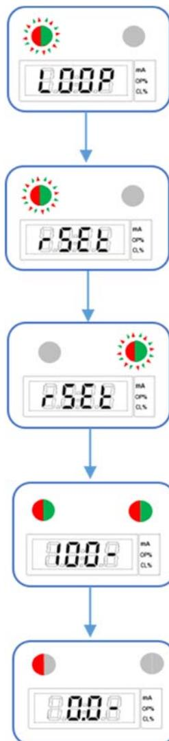
*Figure M: Device Reset*
