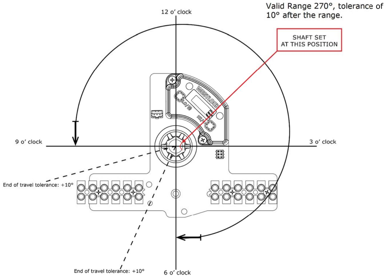
Figure V: Non Contact Sensor – With Solenoid
