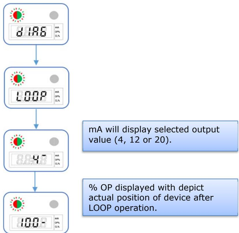
Figure L: Loop Test
