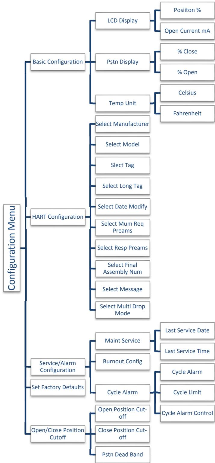
Figure AB: D200 Configuration
