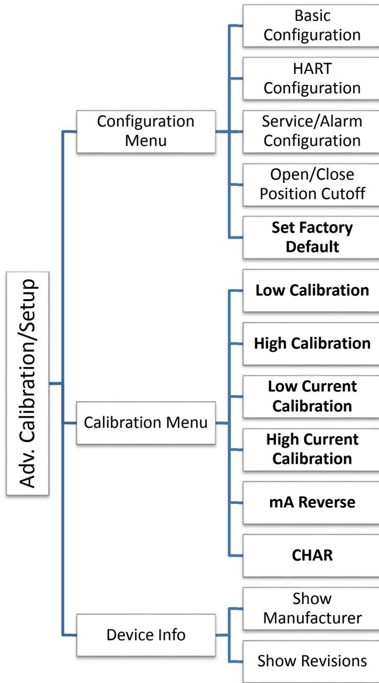
Figure AA: D200 Calibration/Setup
