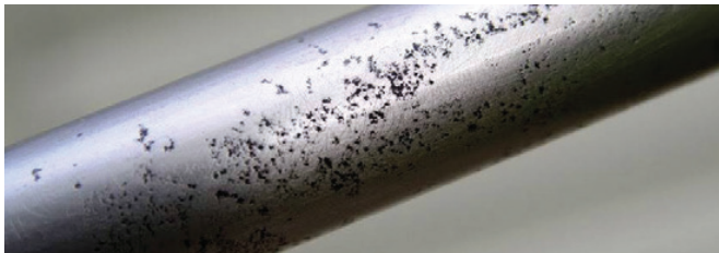
Pitting on Stainless Steel tube after 3 years' service.
