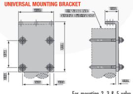
For mounting 2, 3 & 5 valve manifolds to a 2" NB pipestand. Mounting brackets supplied with "U" bolts, washers and nuts. Material of all components is zinc plated and passivated Carbon Steel. Special brackets can be supplied on request.
