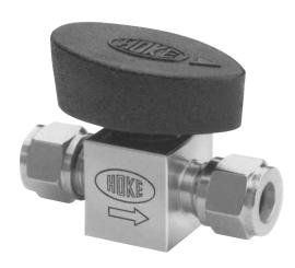
The HOKE® 7300 Series Plug Valve provides full flow or leak-tight shut off with just a quarter turn. The 7300 is recommended for use in applications where instant on-off and visual flow indication is essential. Its safe, reliable top- loaded design allows throttling of fluids and thru-port rodding of the valve. The simple design provides easy maintenance and extends valve life.
