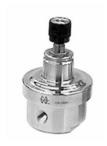
The PR-7ULF Series pressure reducing regulator is designed to furnish ultra precise low outlet pressure control to analytical instrumentation. With the combination of the large diaphragm sensing area of the PR-7 Series regulator and a super low flow valve seat assembly, pressure control down to 1 inch of water at 2cc of flow is easily obtainable.
